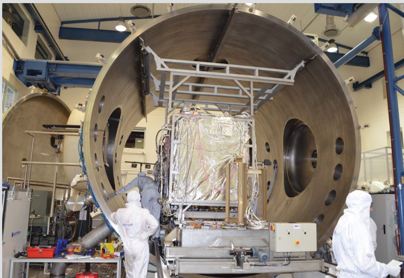
Sentinel-2 Multispectral Instrument ready for thermal vacuum qualification testing at CSL, Belgium (Airbus Defence & Space)
