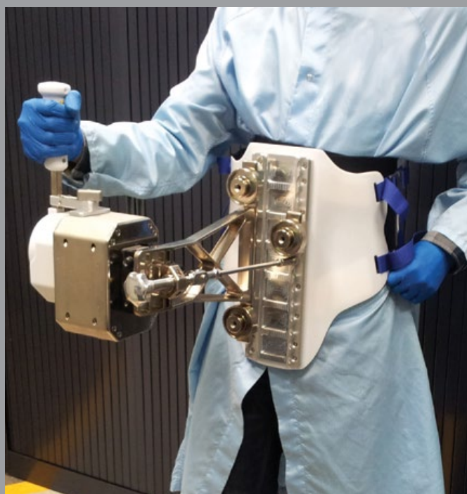
A body-mounted joystick for the Haptics-1 experiment, developed by ESA as part of the multi-agency Meteron initiative, investigating telerobotics for space. The Haptics-1 experiment will be flown to the Space Station on ATV-5 this summer
