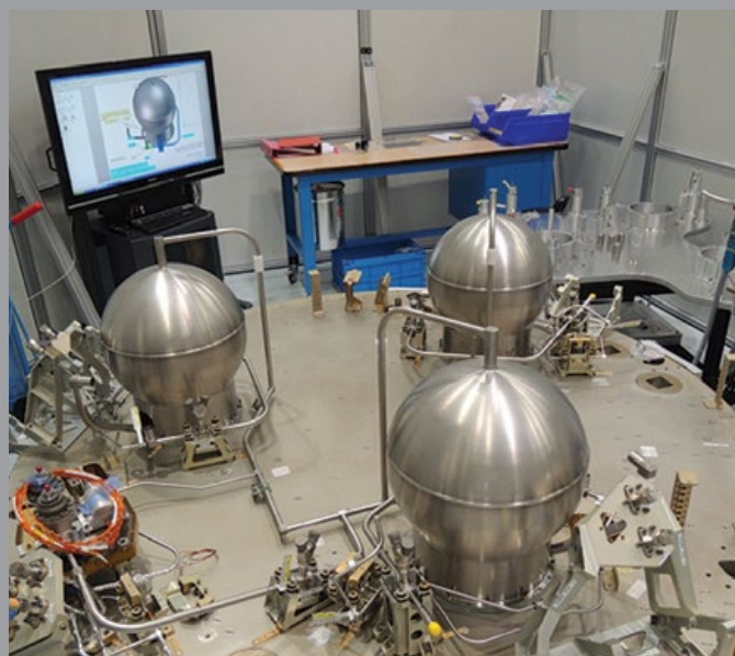
Schiaparelli Flight Model landing platform with integrated propulsion elements (Thales Alenia Space Italy)
