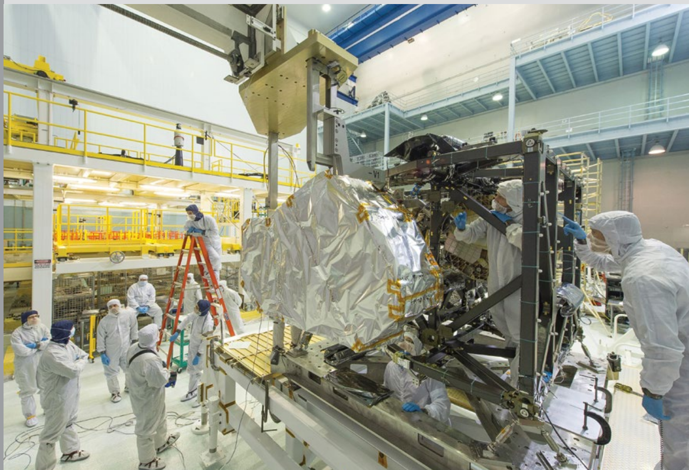
Integration of NIRSpec onto the Webb ISIM Flight Model (NASA)
