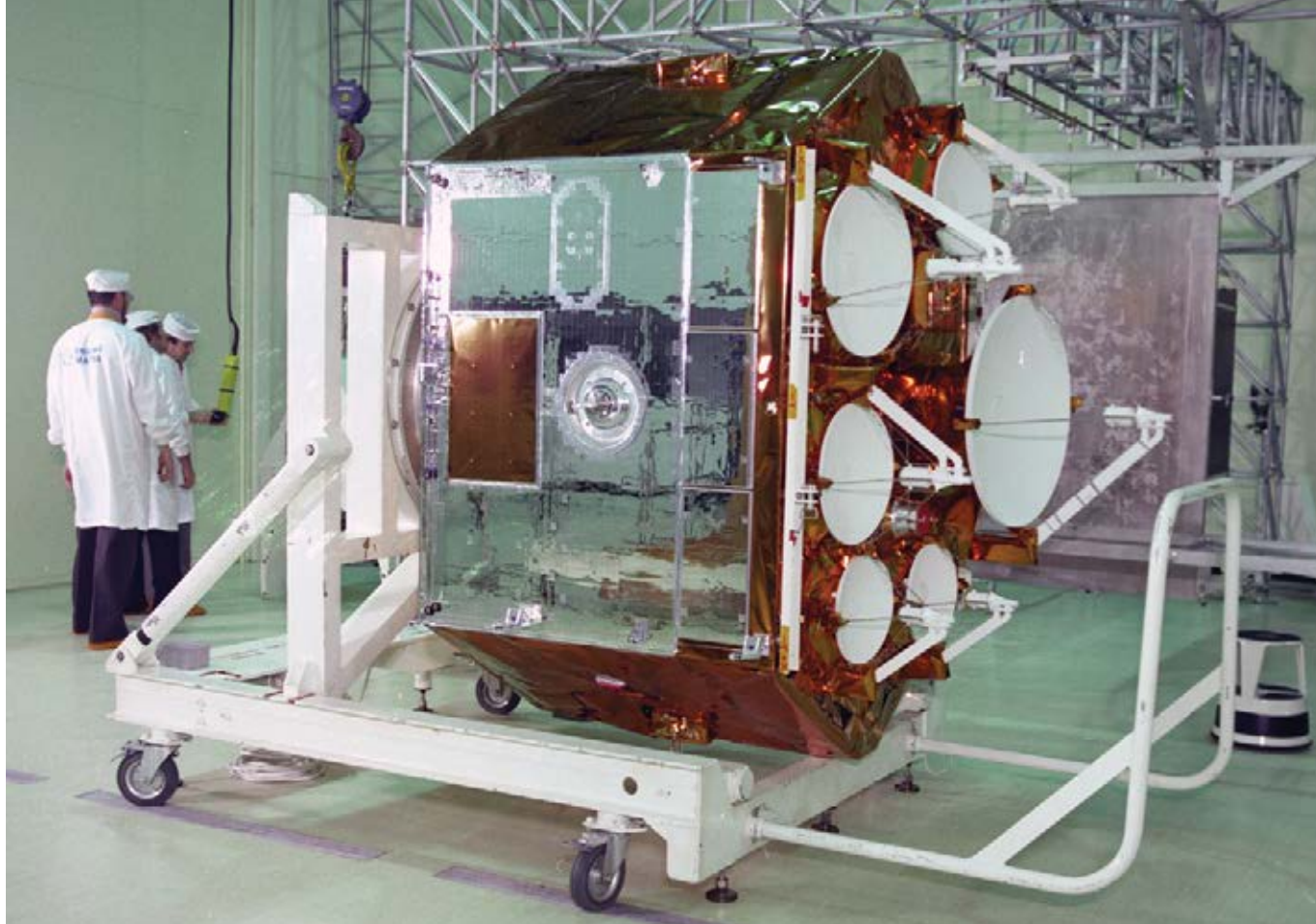
↑ ESA's first telecommunications satellite OTS-2 in the clean room at Matra Toulouse during preparation for testing
