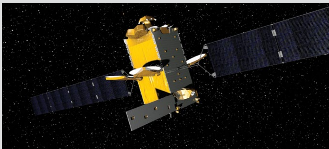
An Alphasat-based telecommunications satellite, with deployable panel radiator to increase thermal rejection capability (Airbus Defence & Space)
